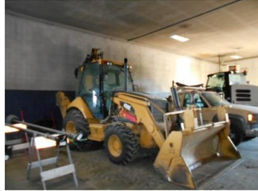
**Existing Condition:** Fair, lot of Hours because of the age of this equipment the out riggers is starting to lose air compression which can become a safety issue.
